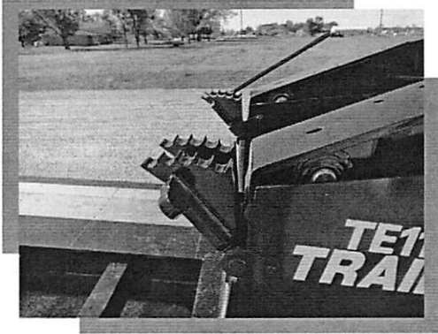
Adjustable transport doors for 5 position deck height.
